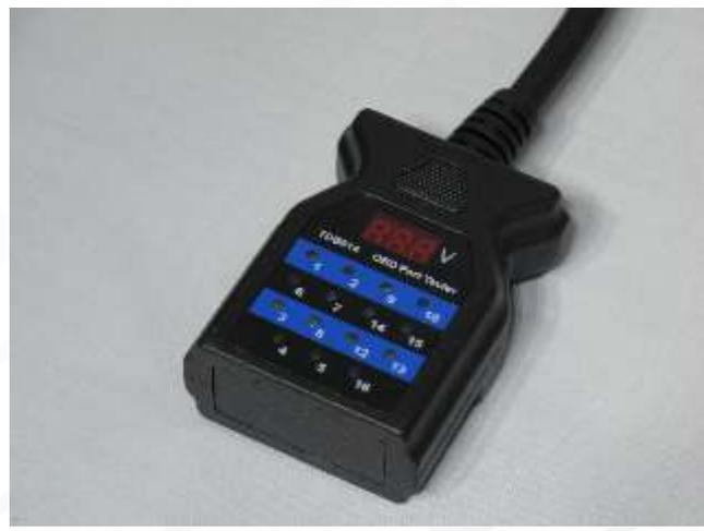
The OBD Port Tester connects to a vehicle's OBDII / EOBD connector and lets you easily diagnose electrical faults.
