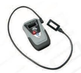
The TDB006 Transponder Antenna Tester has been designed to offer a fast and easy way of checking the transponder antenna across all vehicle systems and types.
