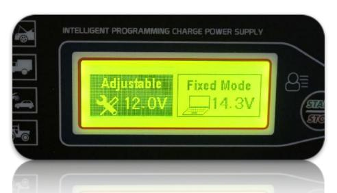
TO ADJUST THE VOLTAGE IN ADJUSTABLE MODE PRESS THE **RIGHT** AND **DOWN** BUTTONS TOGETHER TO ENTER ADJUSTMENT MODE.
